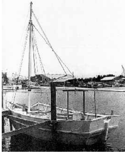
Duchess tied up at a dock in Tarpon Springs. Note the bulwarks, or gunnel, cut out near the bow. The owners intentionally modified Duchess to make it easy for sponge hookers to move around on the deck. (flheritage.com/facts/reports/places/Sites/8PI01704_duchess.cfm).
