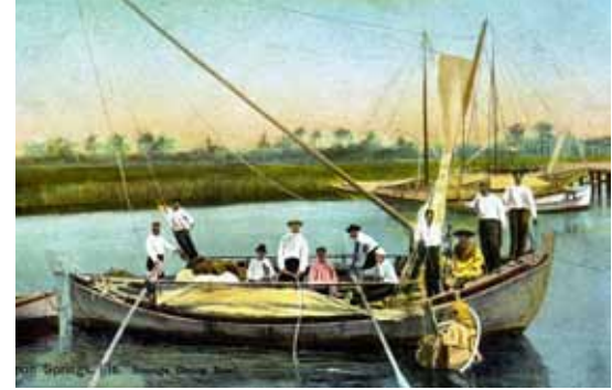
A traditional sponge diving boat, or sacoleve, exhibits the design elements that typified many of the first sponge boats to arrive in Tarpon Springs. Note the double ends and very little freeboard. This type of boat was well-suited for the use of oars. The sailing rig used on the original sponge boats was a sprit mainsail and a forestaysail set to the stem. State Archives of Florida, Florida Memory ( floridamemory.com/items/show/162573 ).
