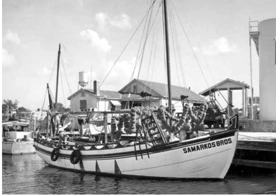
The modern Tarpon Springs sponge boat has retained many of the traditional characteristics of the original sacoleve type. The changes that can be noted in this photograph include the mainmast, which now supports a gaff type mainsail, and the addition of a jigger mast located at the stern. Boatbuilders also modified the stern with a squared transom to incorporate engine power. State Archives of Florida, Florida Memory ( floridamemory.com/items/show/78666 ).
